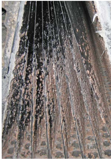
Headbox treated with a competitive biocide after eight weeks (left) and same headbox treated with the Spectrum XD3899 microbiocide after eight weeks (right).
