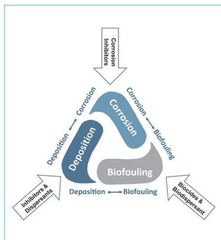
Figure 1 – The cooling water triangle
