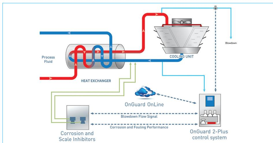
Figure 2 – OnGuard 2-plus control system & OnGuard 3H working principles
