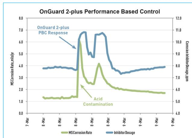
Figure 4 – Monitoring KPIs with OnGuard 2-plus control system
