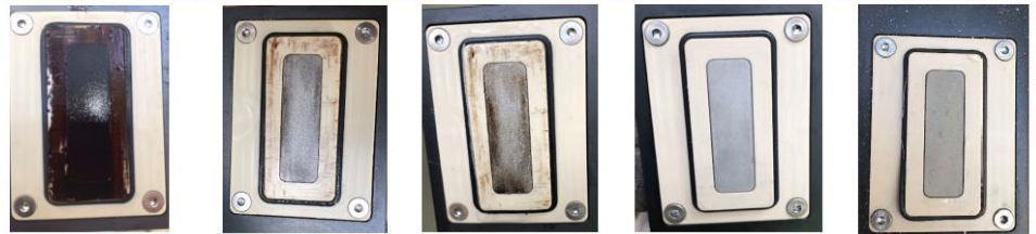
Reduced Manganese Deposition on Probe
