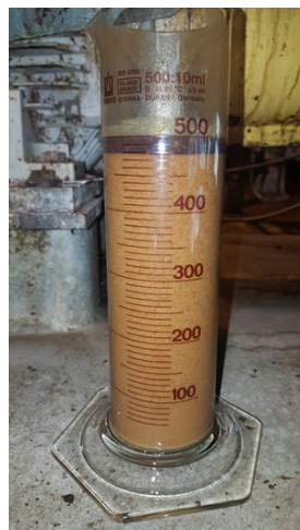
Figure 1: Brine sample, untreated contains tall oil
