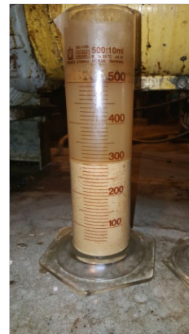
Figure 2: Brine sample, treated with Infinity PS3040E, only spent acid and CaSO 4
