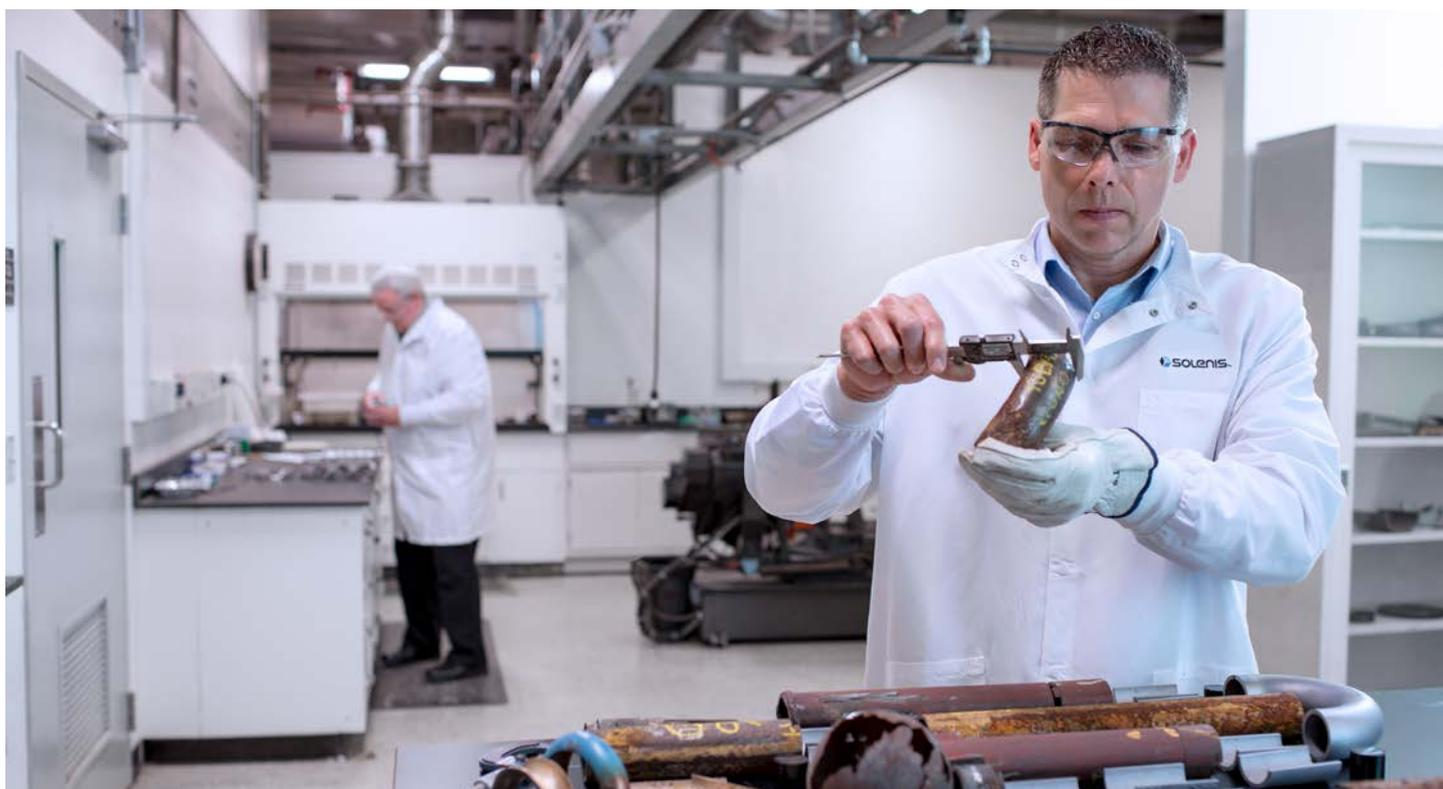
house microbiological, water and deposit analysis laboratories enables a rapid and complete profile of microbiologically influenced corrosion failures.
