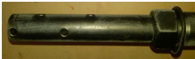
Figure 1: Coupon exposed to Ameroyal 710 Treatment.
