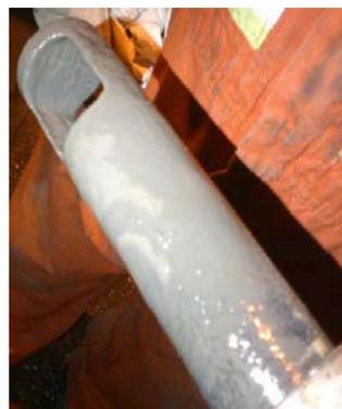
**Soft, easily removable deposit at 40-50 ppm of Zalta 11-440 antiscalant**
