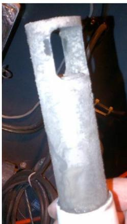
**Scale on probe during competitive trial; difficult to remove**
