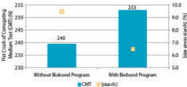
**Figure 4:** Fluting Production: Increased Corrugating Medium Test (CMT) and Reduced Starch Concentration
