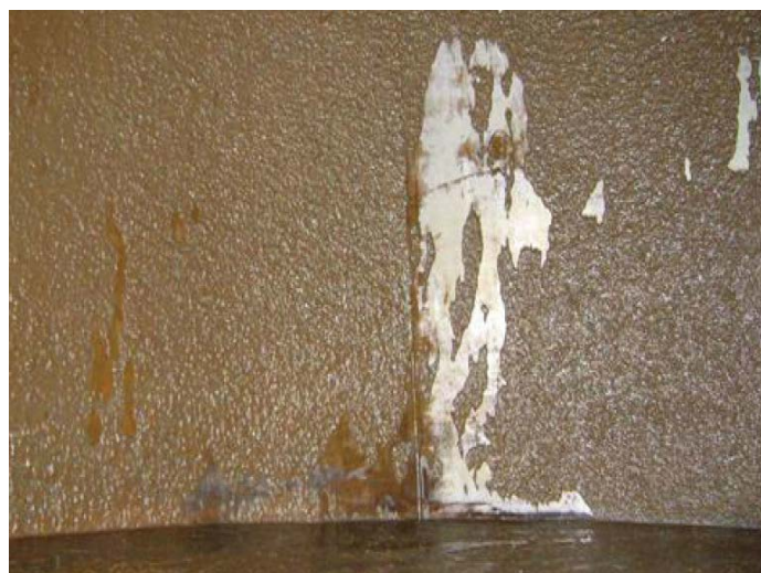
Without the Biobond Program: walls of whitewater chest show high levels of deposition
