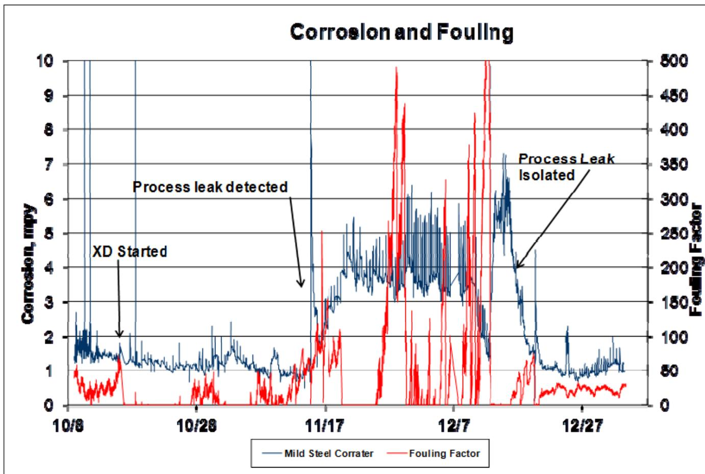
Solenis' OnGuard 2-plus control system detected an increase in corrosion and biofouling caused by a then unknown hydrocarbon leak. Biofouling and corrosion were then controlled to acceptable levels with Biosperse XD3899 microbiocide until a scheduled shutdown could isolate and repair the process leak.
