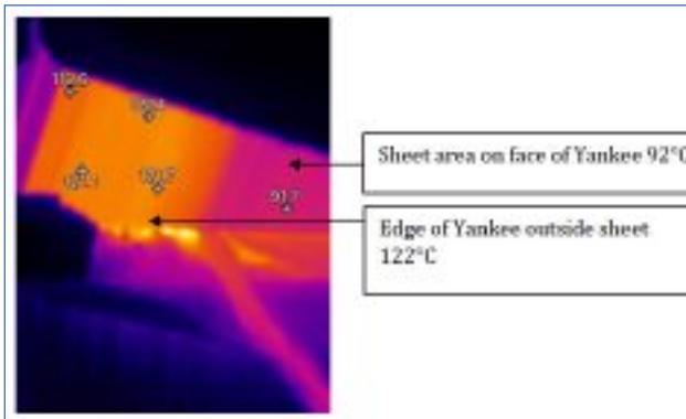
Figure 2: Temperature variation at edge of Yankee cylinder
