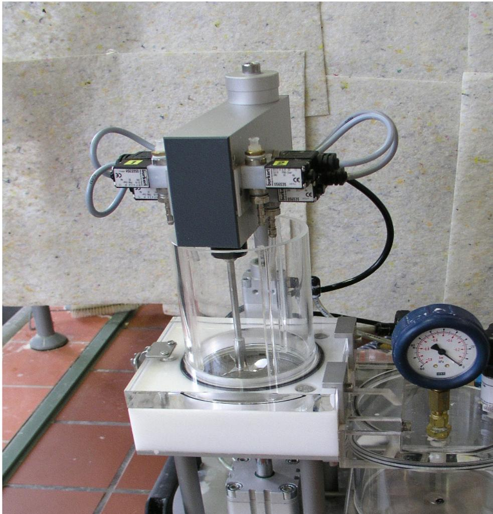
Figure 1. Dynamic Drainage Analyser (DDA)
