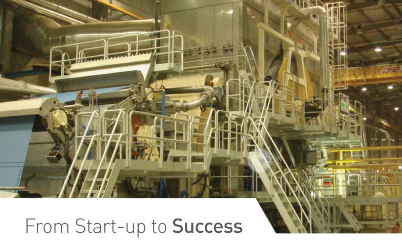
Once a chemical program is determined, Solenis works with mill staff to test it for performance and runnability on the new machine. This involves evaluating the machine's overall functionality, tuning settings on distributed controllers and establishing recommended dosing rates. The testing can last several weeks or even months, but enables the start-up team to analyze the paper for multiple end-use properties and finalize formulation and grade specifications.
