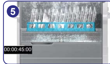
5 Start wash cycle for 45 seconds. Recommended washing temperature is 55 deg c minimum.
