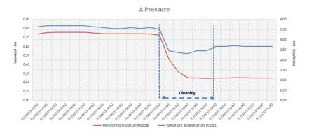
Delta pressure drops after the GeoSol online well cleaning program was performed.
